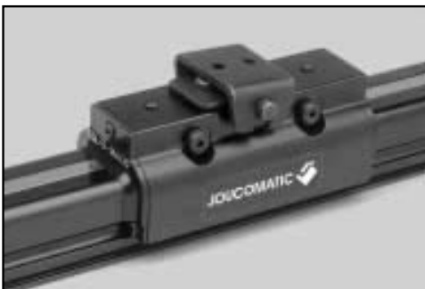
⑤ Carrier with floating mount bracket, alignment compensation for external guided load movement
