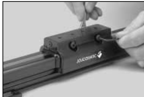
④ Guide adjustment. For heavy duty use, we recommend regularly checking the bracket adjustment
